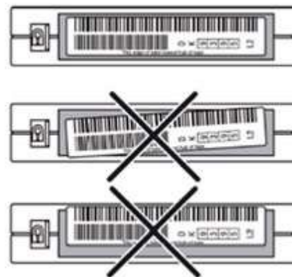
Figure 19 Proper barcode label placement
