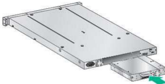
Figure 17 Install a tape drive
