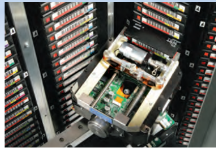
In just 21" of horizontal travel the XLS robot can access over 3,200 tapes insuring fast access times and high reliability
